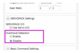
When disabled, return to enable after wiring.
