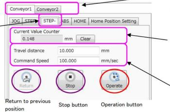
When one-clicking "Operate" button, operation with amount of 1 time STEP of movement is executed in negative direction. When clicking "Stop" button while operating deceleration to a stop is executed.
