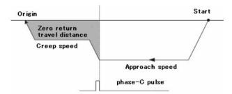
Execute positioning to 0 position for absolute encoder motor.
