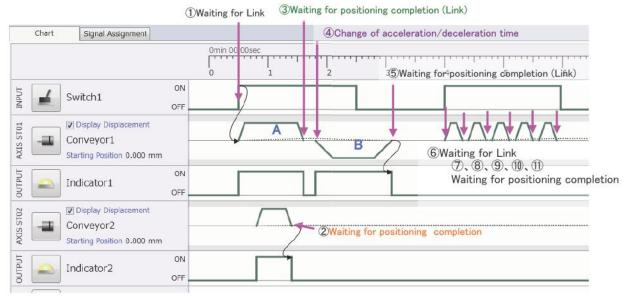
In time chart as shown above, total number of point, that time counter is stopped by MA controller, is 10. The sum, delay of communication and processing are causes of difference from actual time.
