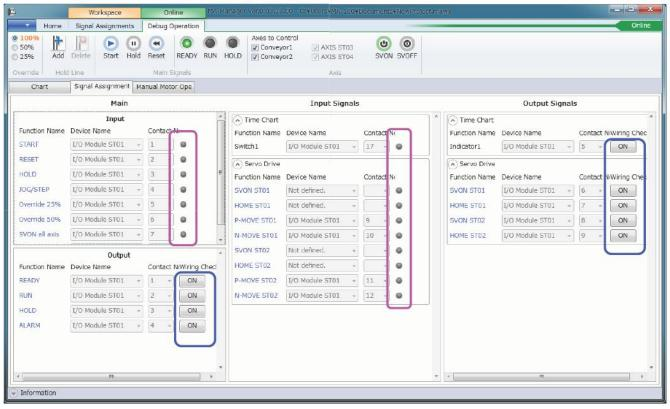
When input signal turns on, the lamp next to the contact number turns on.
