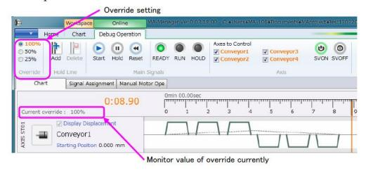
Speed override can be set up with 100%, 50% and 25%.
