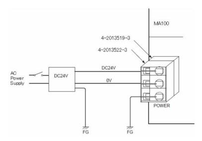
Notes) Using the isolated type power supply DC24 V, and please attach the switch at AC line. 40A inrush current flows when you atached the switch at DC line.
