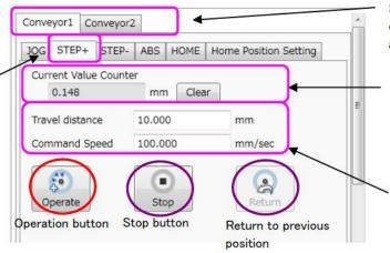
When one-clicking "Operate" button, operation with amount of 1 time STEP of movement is executed in positive direction. When clicking "Stop" button, deceleration to a stop is executed.
