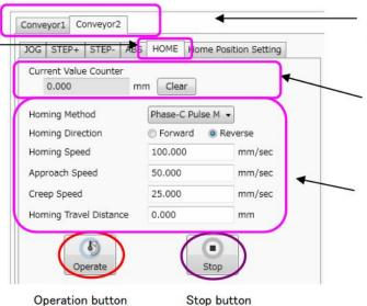
When clicking "Operate" button, zero point return starts. When clicking "Stop" button while operating, deceleration to a stop is executed.
