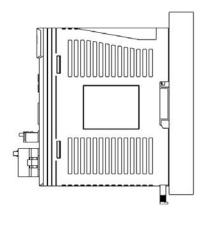
4. Push back DIN rail installation clip, and lock.
