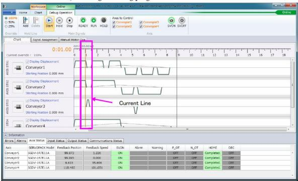
\*\*Current program execution line (Current Line) is at the end line position when operation is completed. Click "Reset" button to return the Current Line to start position of program.
