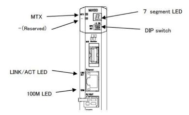
LED that is displayed the motion and abnormality status of Motion Adapter is shown below.
