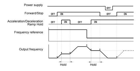
Fig 6.36 Acceleration/Deceleration Ramp Hold
