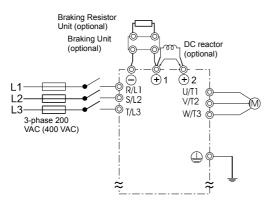
Be sure to remove the short-circuit bar before connecting the DC reactor.
