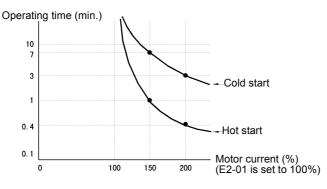
Fig 6.24 Motor Protection Operation Time
