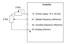
Fig 6.3 Master Speed Frequency Reference Input
