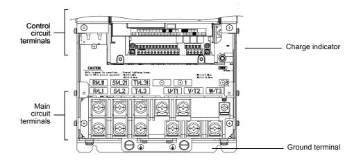
Fig 2.4 Terminal Arrangement (200 V/400 V Class Inverter of 22 kW or more)
