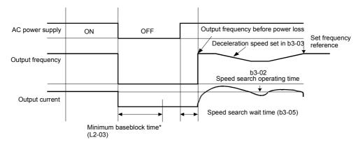
Fig 6.32 Speed Search After Baseblock (Current Detection: Loss Time > L2-03)
