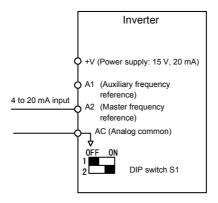
Fig 6.5 Frequency Reference Using Current
