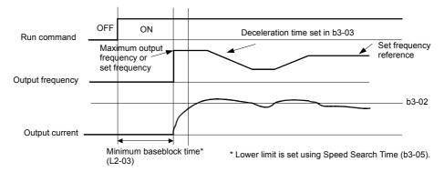
Fig 6.30 Speed Search at Startup (Current Detection)
