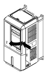
Fig 1.13 Removing the Digital Operator (Model CIMR-E7C45P5 Shown Above)
