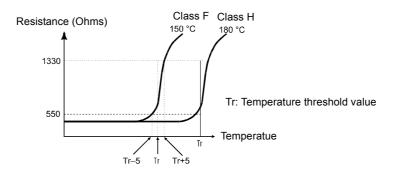
Fig 6.25 PTC Thermistor Temperature-Resistance Value Characteristics\*
