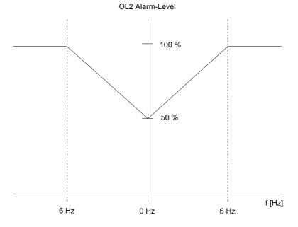
Fig. 6.34 OL2 Alarm Level at Low Frequencies
