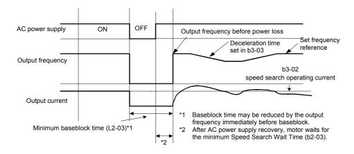
Fig 6.31 Speed Search After Baseblock (Current Detection: Loss Time < L2-03)
