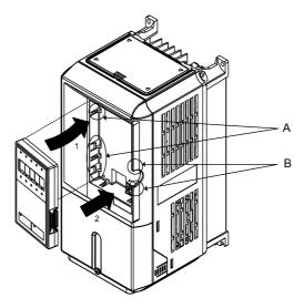
Fig 1.15 Mounting the Digital Operator
