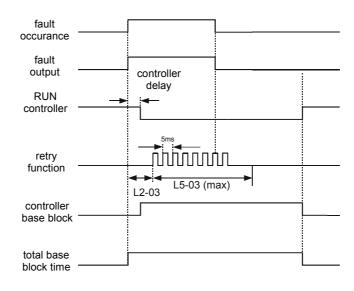
Fig 6.33 Timing Chart for Auto Restart Function
