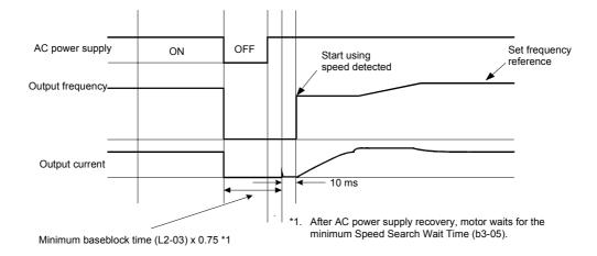
Fig 6.28 Speed Search after Baseblock (Calculated Speed: Loss Time Is Set in L2-03)
