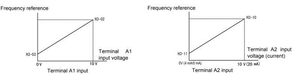
Fig 6.21 Terminals A1 and A2 Inputs
