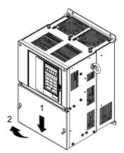
Fig 1.12 Removing the Terminal Cover (Model CIMR-E7C2022 Shown Above)
