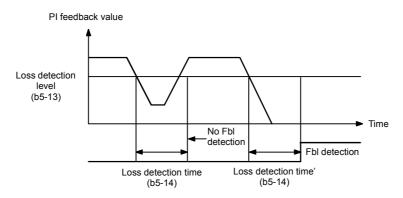
Fig 6.50 PI Feedback Loss Detection Time Chart
