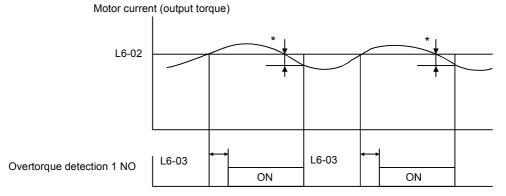
\*Overtorque detection switch off bandwidth is approximately 10% of the Inverter rated output current (or motor rated torque).
