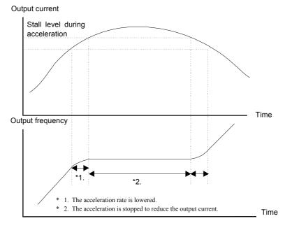
Fig 6.18 Time Chart for Stall Prevention During Acceleration
