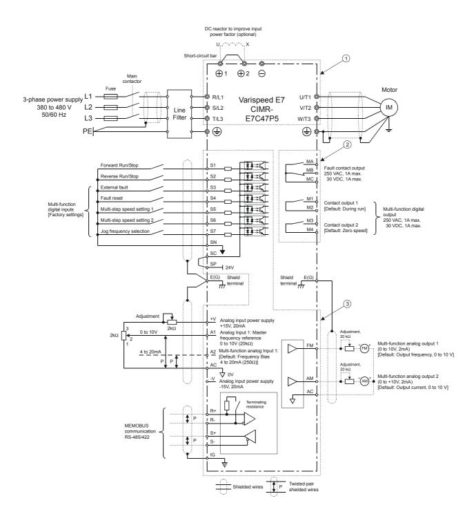
Fig 2.2 Connection Diagram (Model CIMR-E7C47P5 Shown Above)
