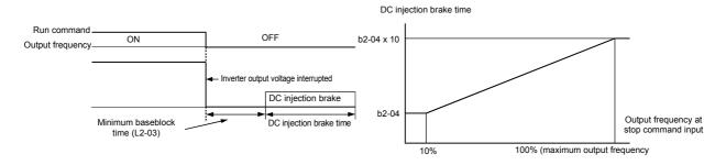
Fig 6.13 DC Injection Braking Stop
