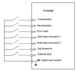
Fig 6.6 Control Circuit Terminal During 5-step Operation
