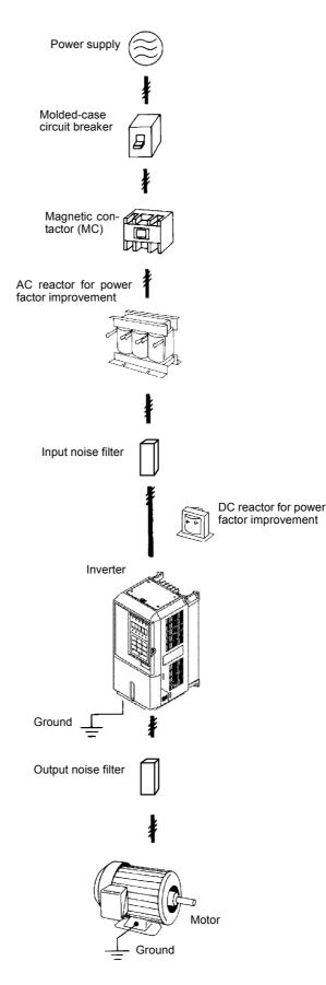
Fig 2.1 Example Connections to Peripheral Devices
