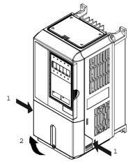
Fig 1.11 Removing the Terminal Cover (Model CIMR-E7C25P5 Shown Above)
