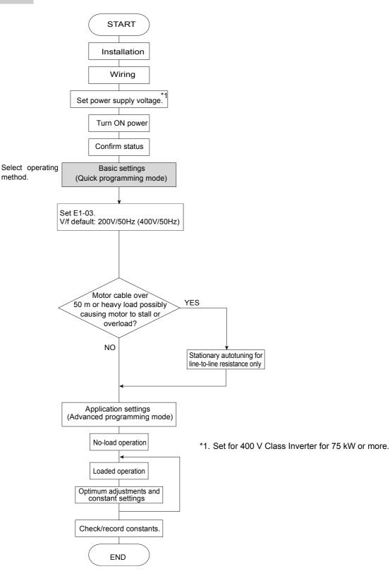
Fig 4.1 Trial Operation Flowchart
