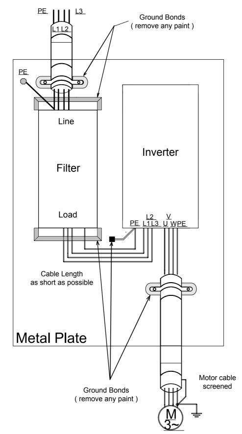
■ Installation inverters and EMC filters
