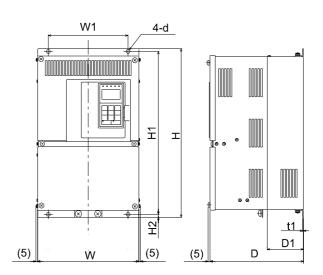
200 V/400 V Class Inverters of 0.55 to 18.5 kW
