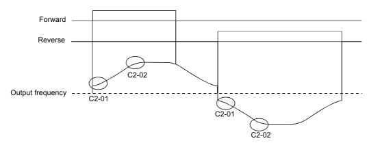
Fig 6.17 S-curve Characteristic during Operation Switching
