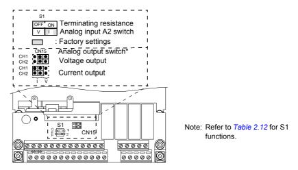
Fig 2.13 Jumper CN15 and DIP Switch S1
