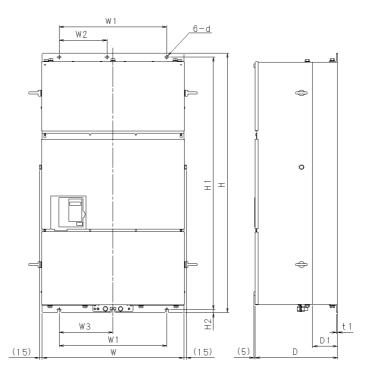
400 V Class Inverters of 185 to 300 kW
