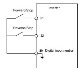
Fig 6.8 2-Wire Control Wiring Example with Positive Logic
