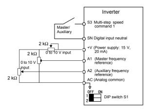
Fig 6.4 Master/Auxiliary Frequency Reference Input
