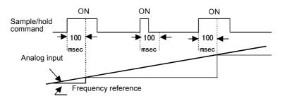
Fig 6.39 Sample/Hold Analog Frequency
