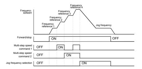
Fig 6.7 Multi-step speed command/Jog Frequency Selection Time Chart
