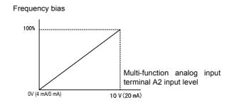
Fig 6.22 Frequency Bias Adjustment (Terminal A2 Input)
