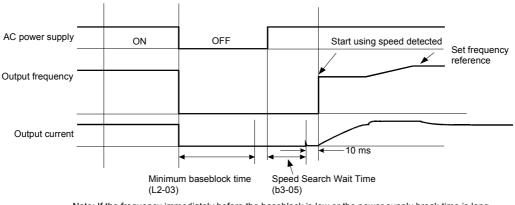
Note: If the frequency immediately before the baseblock is low or the power supply break time is long, operation may be the same as the search in case 1.
