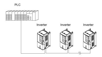
Fig 6.43 Example of Connections between PLC and Inverter
