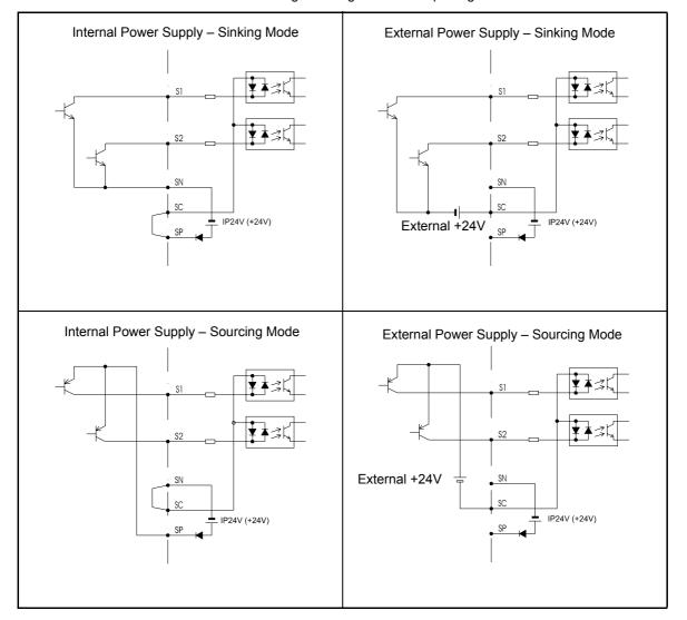
Table 2.13 Sinking/Sourcing Mode and Input Signals
