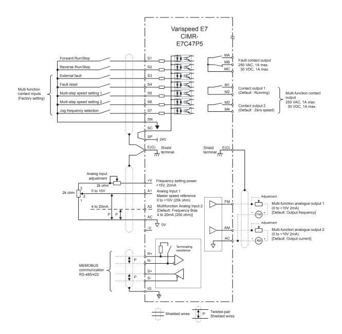
Fig 2.14 Control Circuit Terminal Connections
