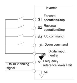
Fig 6.37 Connection Example when UP/DOWN Commands Are Allocated
