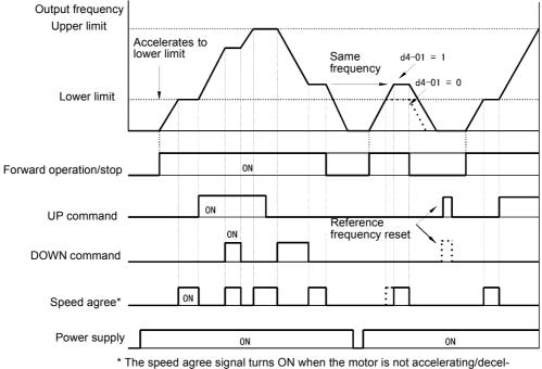
\* The speed agree signal turns ON when the motor is not accelerating/decelerating while the run command is ON.
