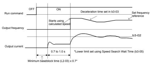
Note: If the stopping method is set to coast to stop, and the run command turns ON in a short time, the operation may be the same as the search in case 2.
