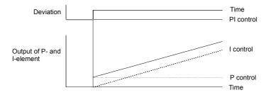
Fig 6.48 PI Control Operation
