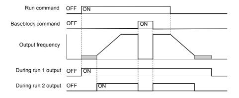
Fig. 6.40 Timing Chart for "During RUN" Output
