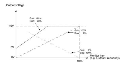
Fig 6.42 Monitor Output Adjustment
