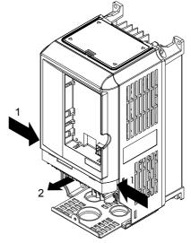
Fig 1.14 Removing the Front Cover (Model CIMR-E7C45P5 Shown Above)
