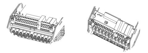
Fig 8.5 Removing the Control Circuit Terminal Card
