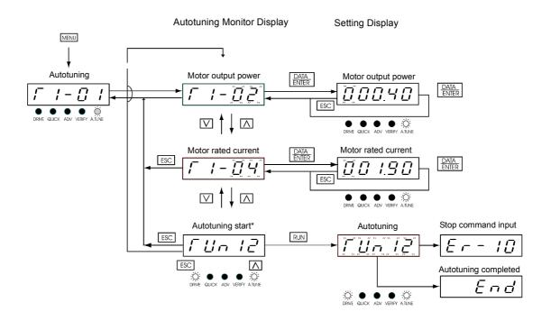
Fig 3.8 Operation in Autotuning Mode
