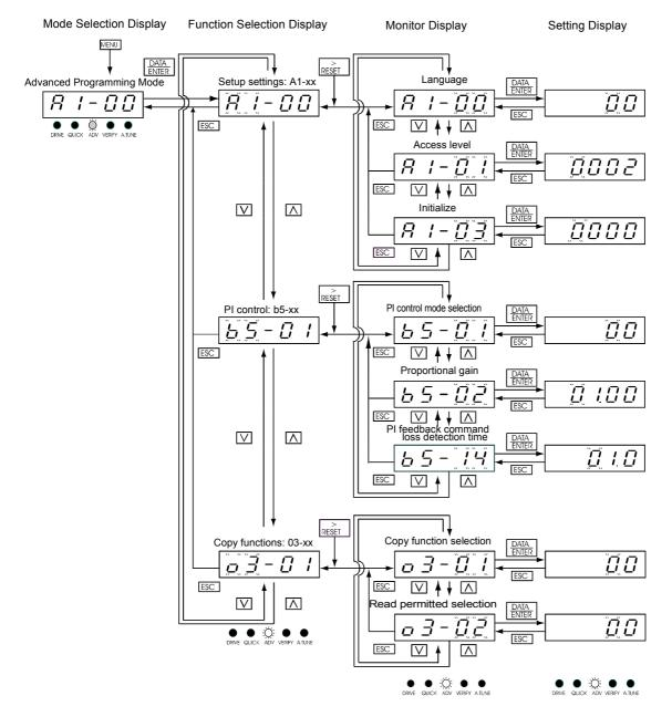
Fig 3.6 Operations in Advanced Programming Mode
