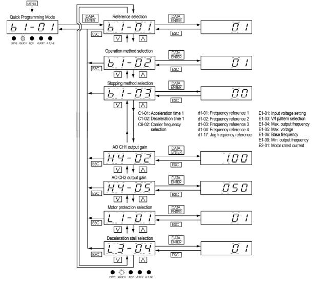
Fig 3.5 Operations in Quick Programming Mode
