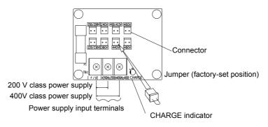
Fig 4.2 Power Supply Voltage Setting
