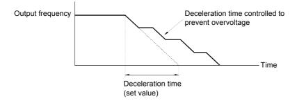
Fig 6.20 Stall Prevention During Deceleration Operation
