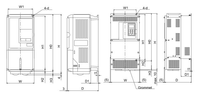
200 V/400 V Class Inverters of 0.55 to 18.5 kW
