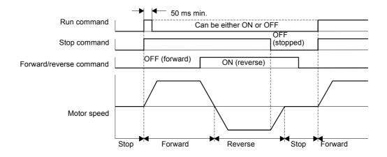
Fig 6.10 Three-wire Control Time Chart
