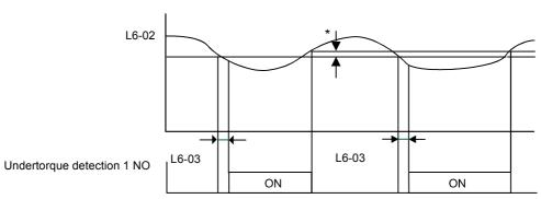
\*Undertorque detection switch off bandwidth is approximately 10% of the Inverter rated output current (or motor rated torque).
