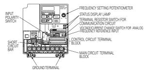
Example of 3-phase (200V class, 1.5kW) inverter
