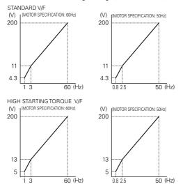
When operating with frequency larger than 60Hz/50Hz, change only max. output frequency (n011).
