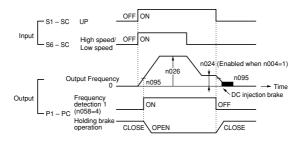
• For a variable speed operation by an analog signal, set the frequency reference selection (n004) to a value from 2 to 4.
