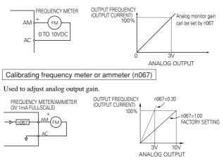
Set the analog output voltage at 100% of output frequency (output current). Frequency meter displays 0 to 60Hz at 0 to 3V.
