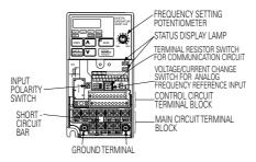
Example of 3-phase (200V class, 0.1kW) inverter
