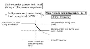
• Stall prevention (current limit) level during running (n094) Sets the stall prevention (current limit) level during running in units of 1%. (Inverter rated current = 100%)
